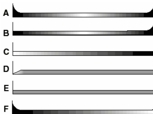
Figure 2-11: Six Patterns of Failure (Mourbrey, 2001)
