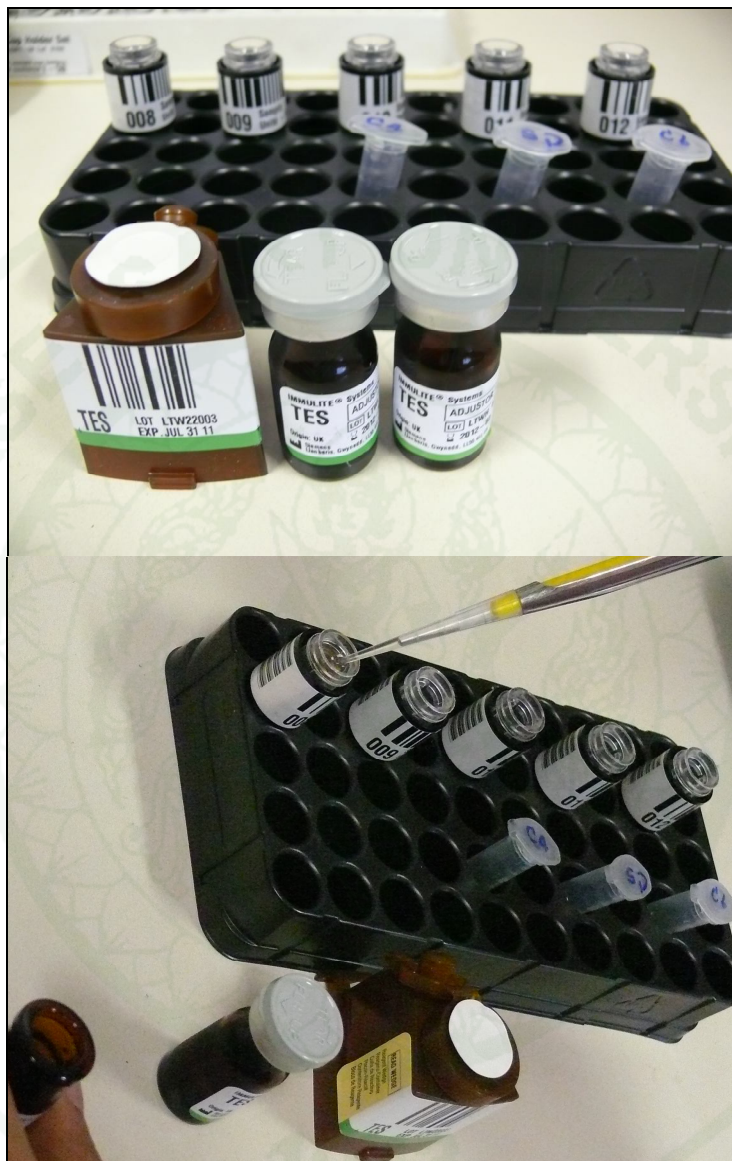
Appendix Figure 19 Immulite™ test kit for serum T measurement by chemiluminescence method.
