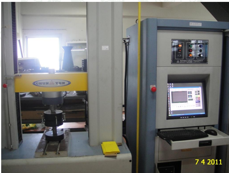
Appendix Figure B8 Testing compressive strength of mortar with Universal Testing Machine
