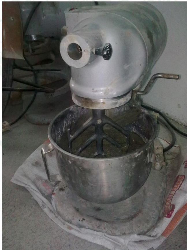
Appendix Figure B6 Mixing mortar
