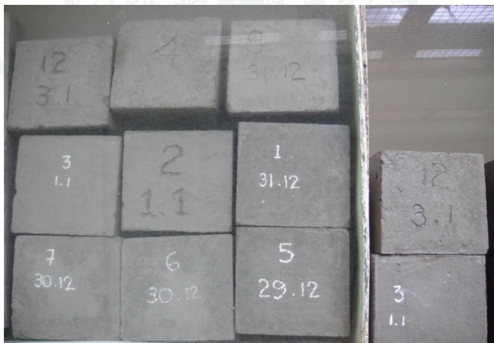
Appendix Figure B2 Curing of specimens in water
