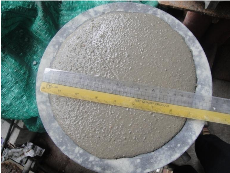
Appendix Figure B7 Measuring flow of mortar
