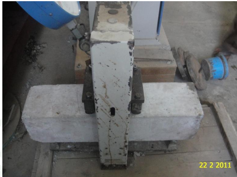
Appendix Figure B5 Testing flexural strength of VA concrete
