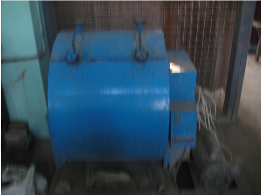
Appendix Figure B3 Testing Los Angeles abrasion
