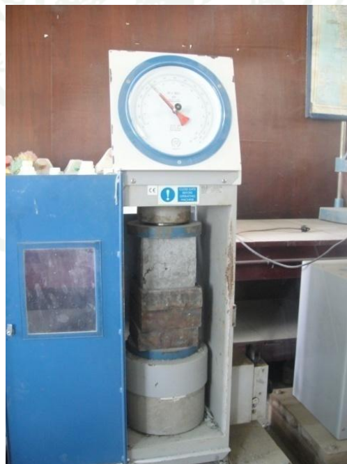
Appendix Figure B4 Testing compressive strength with ELE testing machine
