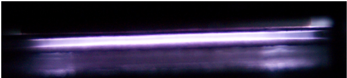
Figure 4.4 Photograph of homogenous argon plasma with bluish pink color.
