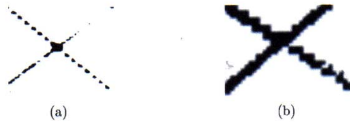
Figure 2.9 Improper thresholding of lines: (a) underthresholding causes corrupted and non-continuous lines. (b) overthresholding leads to lines spanning multiple pixels
