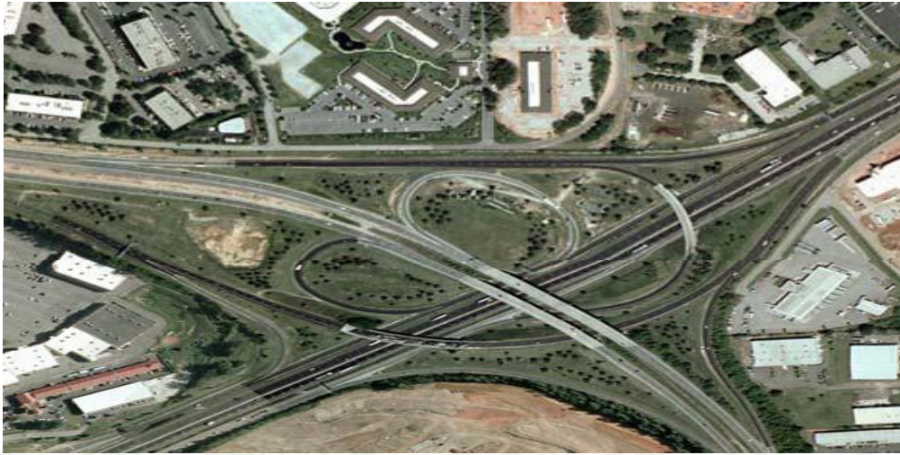
Figure 7 Grade-separated with ramps (interchanges)
