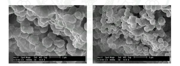
Appendix Figure A3 SEM images of cross-section of C8-silica monolith in the microfluidic chip
