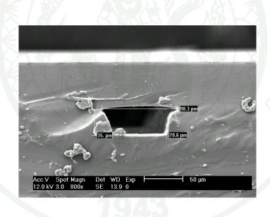
Figure 8 SEM photograph of microfluidic chip.
