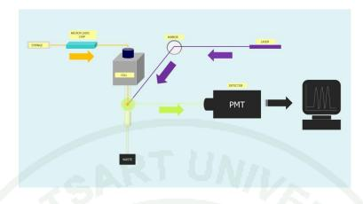
Appendix Figure A2 Schematic of laser-induced fluorescence using determine compounds
