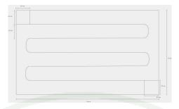
Appendix Figure A1 Configuration of the microfluidic chip
