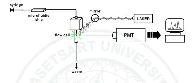
Figure 3 Schematic diagram of the integrated monolith microfluidic chip with LIF instrument
