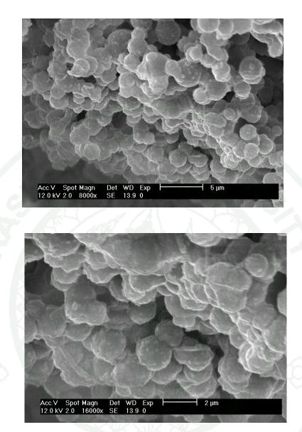
Figure 9 SEM images of cross-section of  $C_8$ -silica monolith in the microfluidic chip
