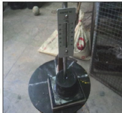
Figure 13 Normal consistency of cement testing by a Vicat needle apparatus
