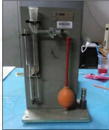
Figure 8 Fineness of cement powders analyzed by a Blaine air permeability apparatus
