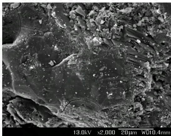
Appendix Figure H9 SEM image of C100B0 at curing times 90 days at x2,000
