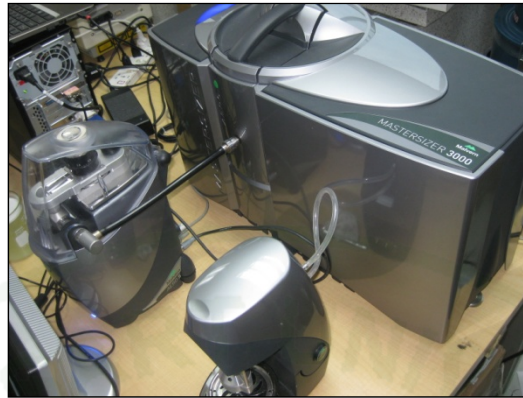
Figure 7 Particles size distribution of cement powders analyzed by a smarter particle sizing
