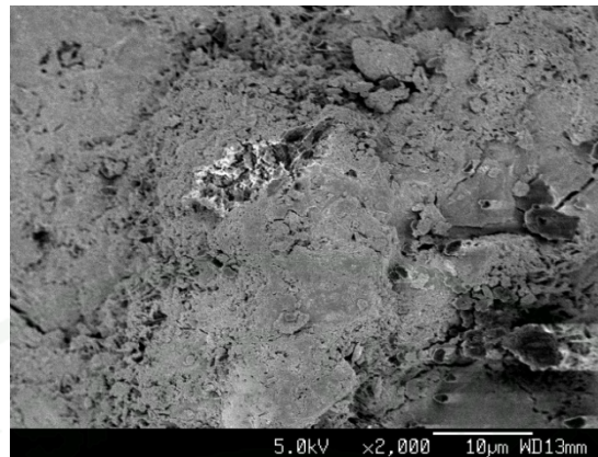
Appendix Figure H11 SEM image of C90B10 at curing times 28 days at x2,000
