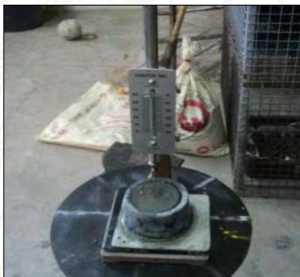
Figure 14 Setting time of cement testing by a Vicat needle apparatus
