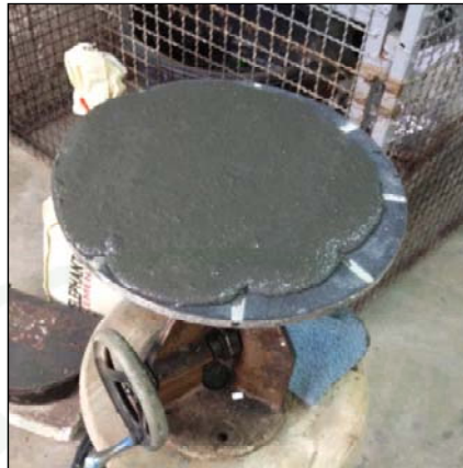
Figure 11 Flowability testing by flow table and flow mold
