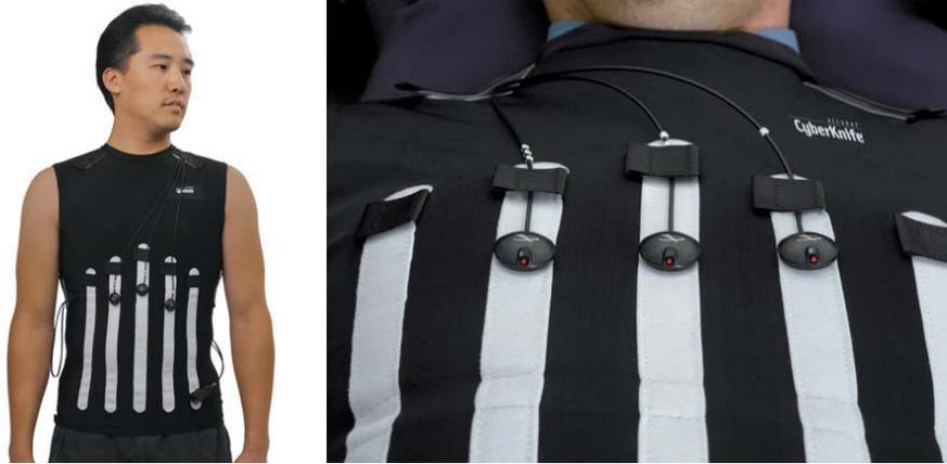
**Figure 3B** Three LED markers are attached to vest that the patient wears during treatment
