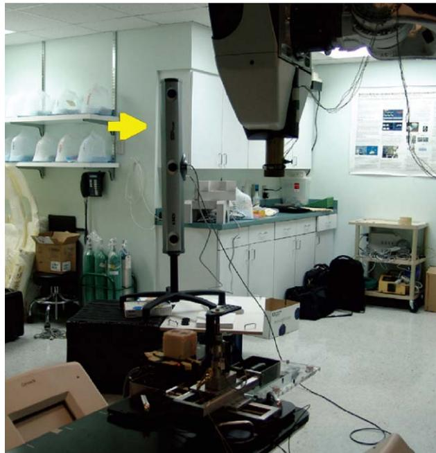
**Figure 3.3** The set up of the Optotrak certus (Arrow) in Cyberknife treatment room. Two LEDs are attached to the tumor motion simulator near the target ball-cube. An additional six LEDs are attached to the final collimator of the Cyberknife Linac.
