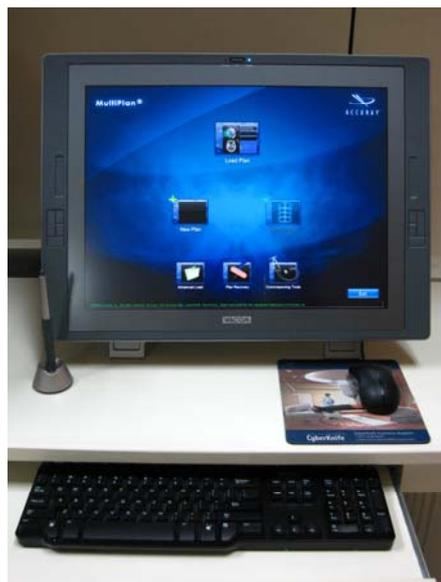
**Figure 4.15** The MultiPlan<sup>®</sup> treatment planning system
