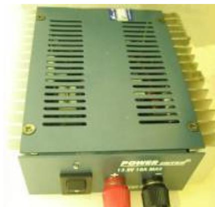
**Figure 4.3** Switching power supply
