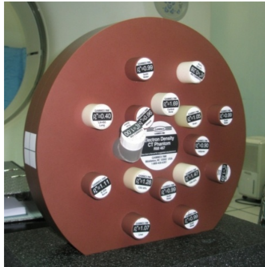
Figure 1.2 Phantom (Gammex RMI 467) for CT calibration which inserted samples of known mass and electron density.
