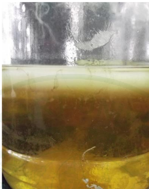
Figure 3 BC pellicle formed in static culture.
