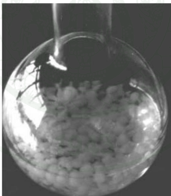
Figure 4 BC pellets formed in agitated culture.
