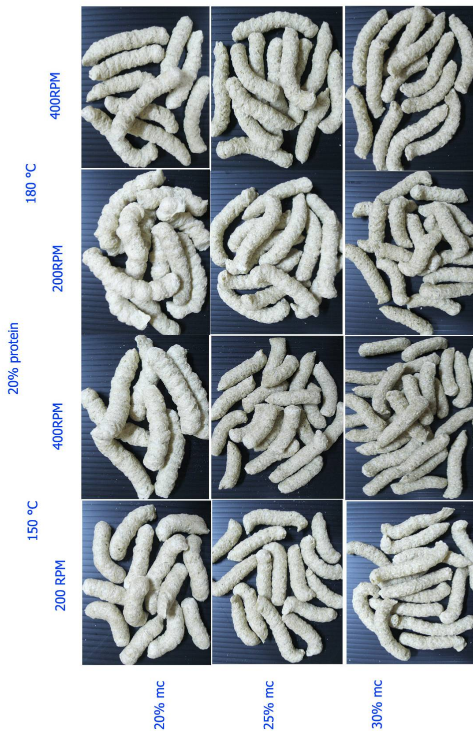
Appendix Figure D1 Non-enrobed of glutinous rice, fish meal, soy and gluten extrudates
