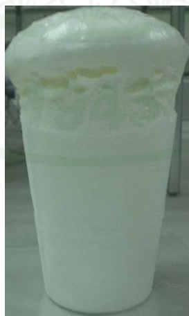
Appendix Figure A33 Foam composite (Zeolite+gel_110/300)
