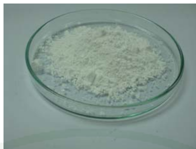
Appendix Figure A26 Calcium Zeolite Type A dried at 110°C (gel_110)
