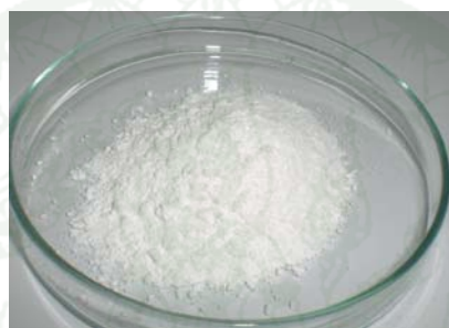
Appendix Figure A27 Calcium Zeolite Type A calcined at 300°C (gel_300)
