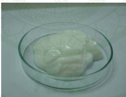
Appendix Figure A25 Calcium Zeolite Type A gel
