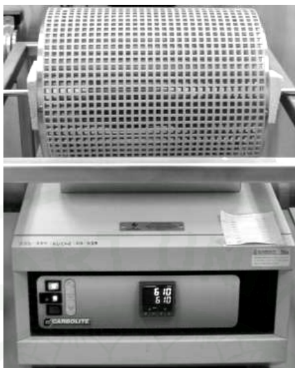
Figure 23 The reactor of methane cracking reaction equipped with the electric heater (Carbolite tube furnace).
