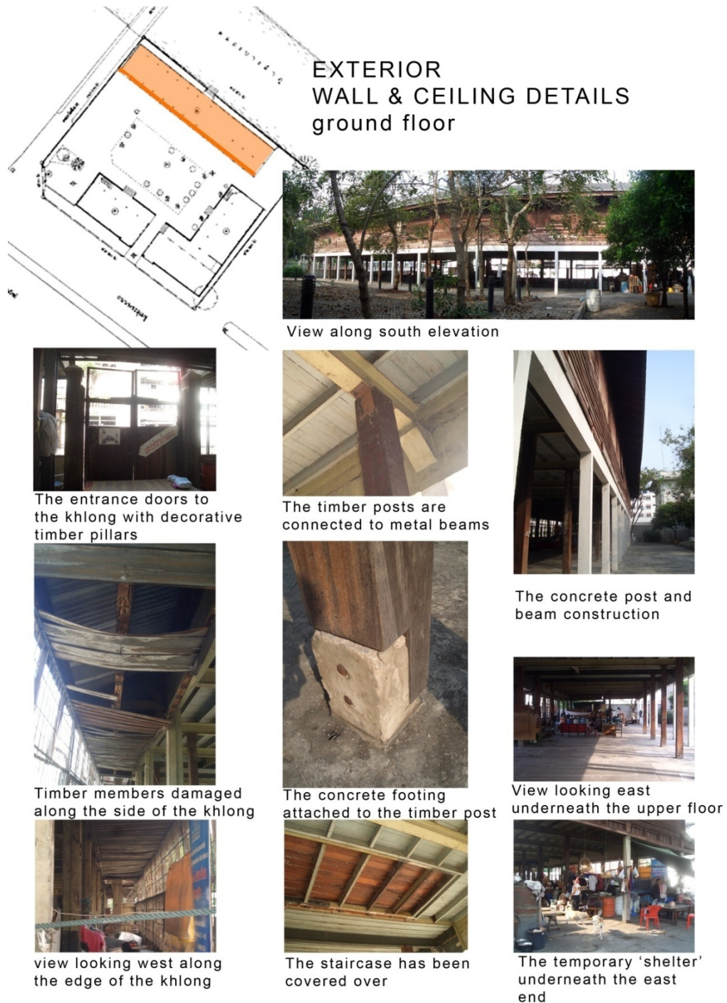
Figure 15 Kuru Sapha - exterior wall + ceiling details (timber building) (author)
