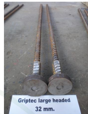
Appendix Figure B7 GRIPTEC Large and small headed bars dia 32 mm
