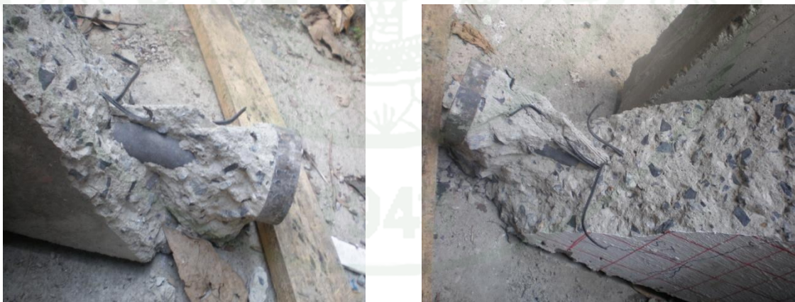
Figure 73 Conical wedge shape behind head surface
