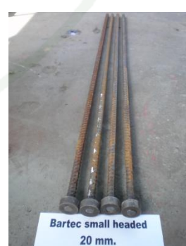
Appendix Figure B9 BARTEC small headed bars dia 20 mm and 32 mm
