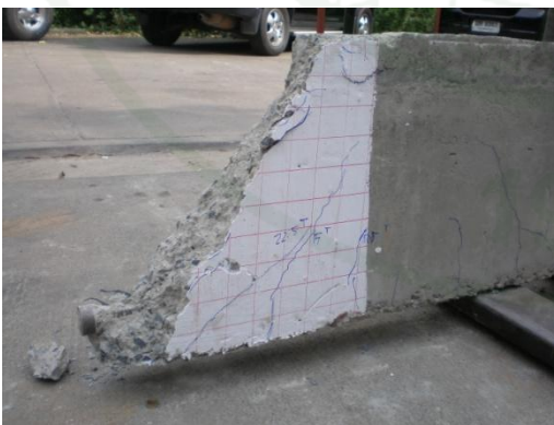
Figure 79 Left top portion cleaved part
