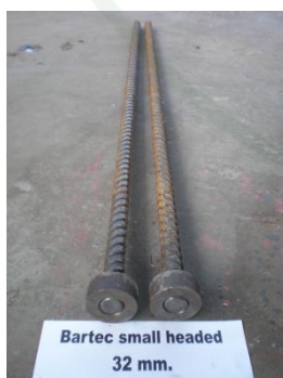
Appendix Figure B9 BARTEC small headed bars dia 20 mm and 32 mm
