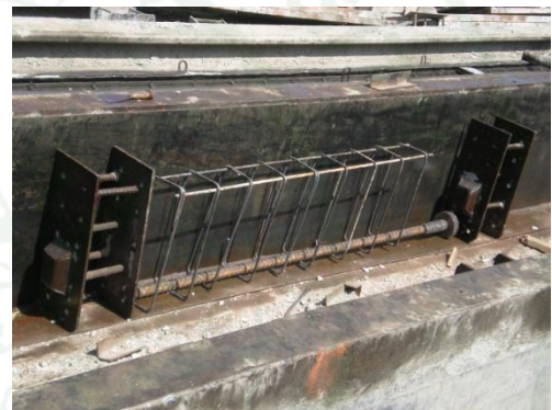
Appendix Figure B16 Strain gauge installation along bars
