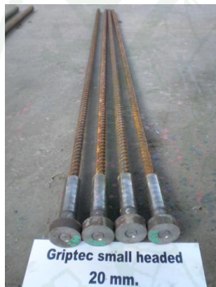
Appendix Figure B8 GRIPTEC Large and small headed bars dia 20 mm
