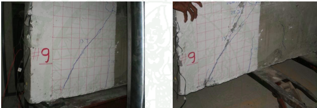
Appendix Figure B38 Cracking behavior for U-20-320-4.32-B-1/1
