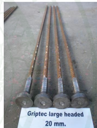
Appendix Figure B8 GRIPTEC Large and small headed bars dia 20 mm
