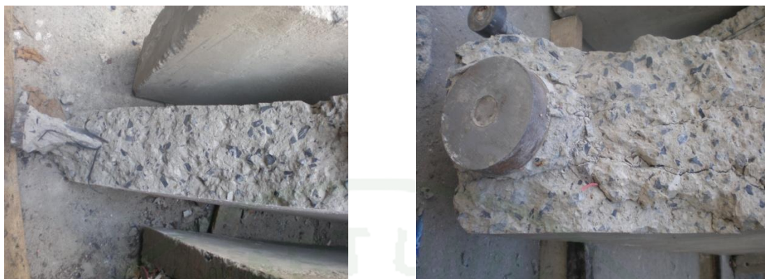
Figure 74 Conical wedge shape behind head surface
