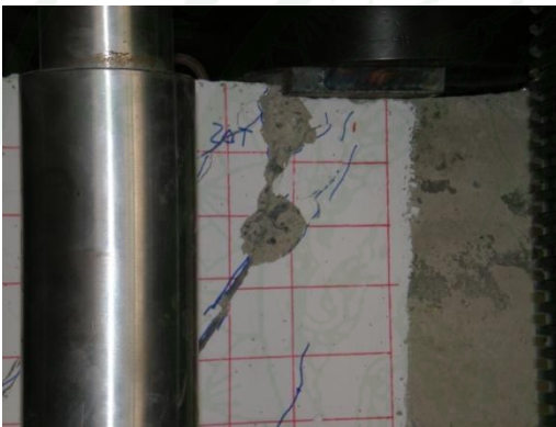
Figure 78 Diagonal cracked plane
