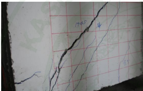
Appendix Figure B32 Cracking behavior for U-20-240-9.59-G-1/1
