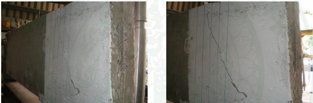
Appendix Figure B44 Cracking behavior for U-20-320-0.00-H-1/1
