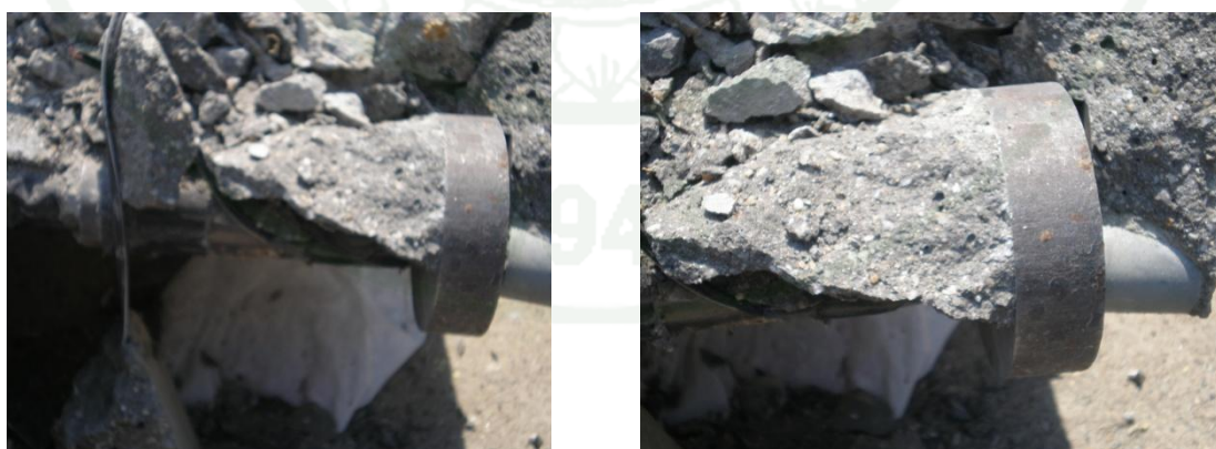
Figure 76 Conical wedge shape behind head surface
