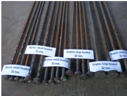
Appendix Figure B10 BARTEC and GRIPTEC large and small headed bars dia 20
