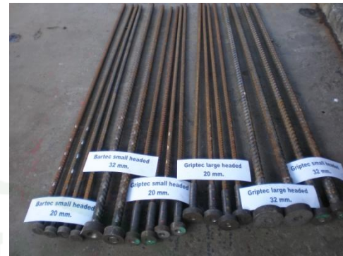
Appendix Figure B10 BARTEC and GRIPTEC large and small headed bars dia 20
