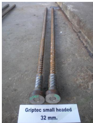
Appendix Figure B7 GRIPTEC Large and small headed bars dia 32 mm
