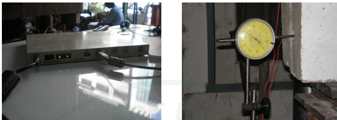
Figure 45 Data logger and dial gauges
