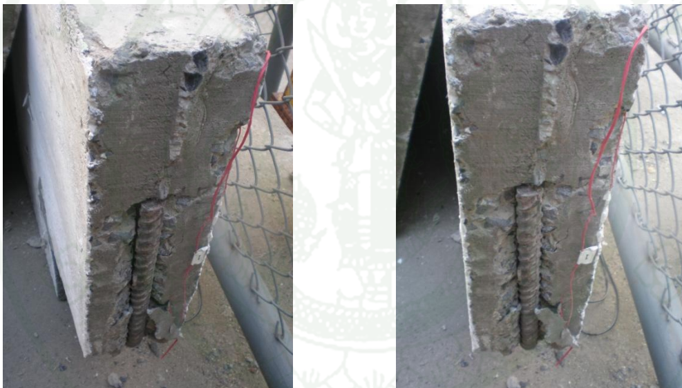
Figure 81 Spall failure of 90° hooked bar
