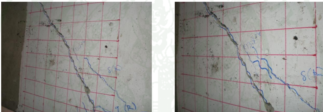
Appendix Figure B35 Cracking behavior for U-20-240-4.10-G-1/2
