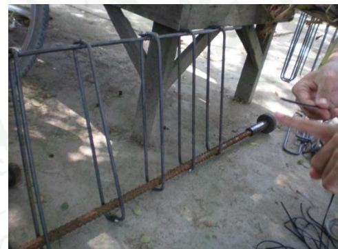
Appendix Figure B10 BARTEC and GRIPTEC large and small headed bars dia 20
