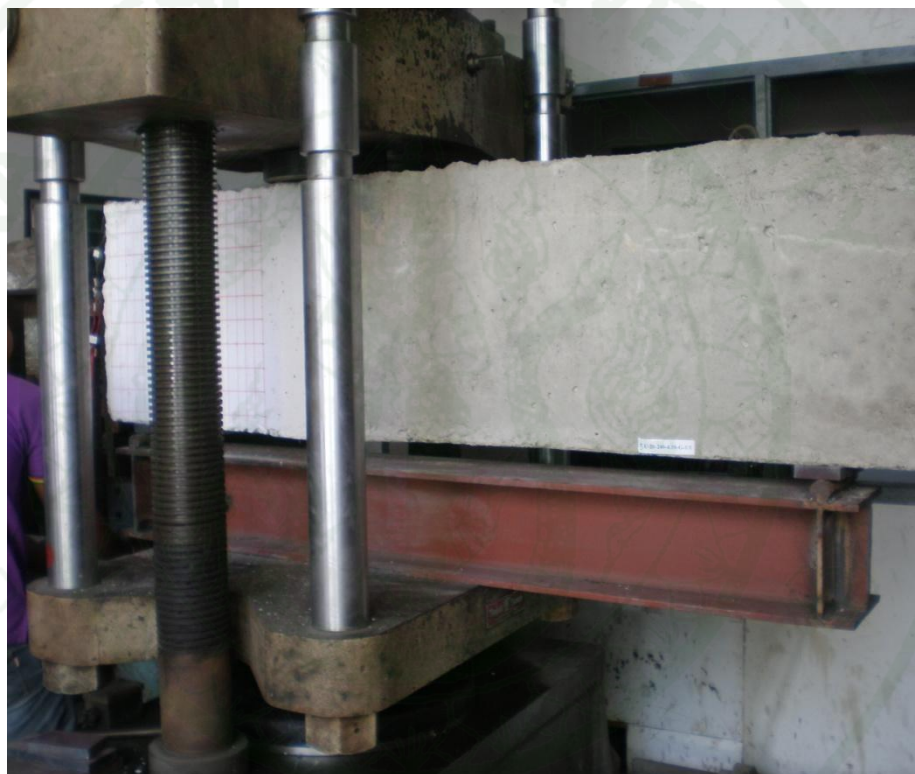
Figure 37 A typical CCT node test
