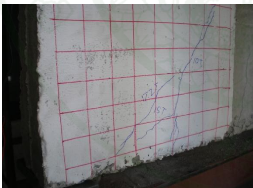
Appendix Figure B33 Cracking behavior for U-20-240-9.59-G-1/2
