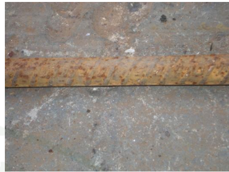
Appendix Figure B1 Dia 20 mm and 32 mm control bars SD40
