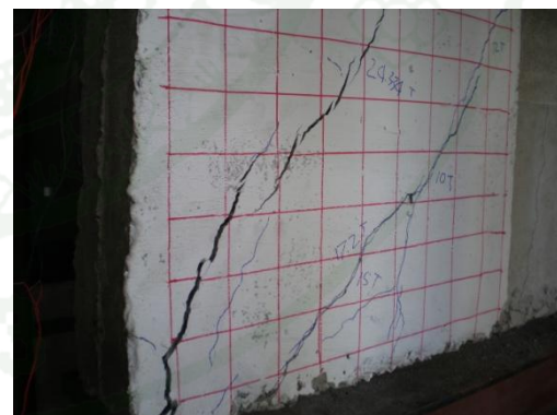
Appendix Figure B33 Cracking behavior for U-20-240-9.59-G-1/2
