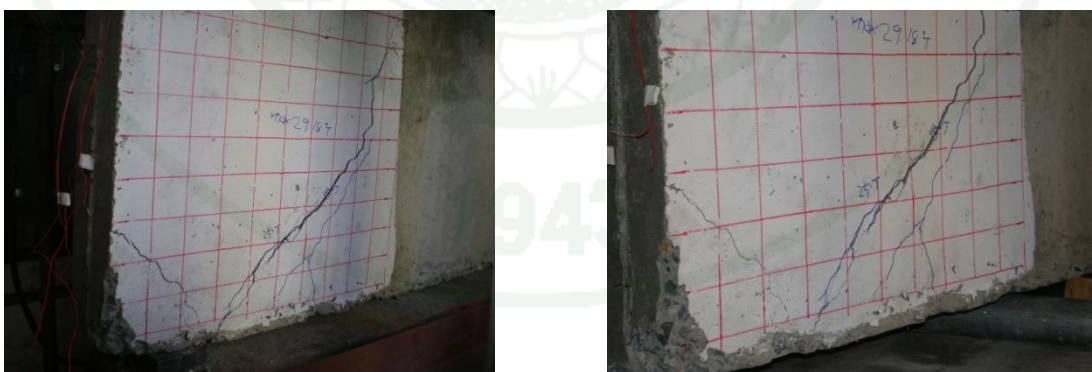
Appendix Figure 45 Cracking behavior for U-20-320-0.00-H-1/2
