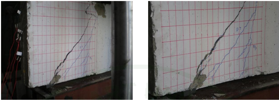
Appendix Figure B34 Cracking behavior for U-20-240-4.10-G-1/1
