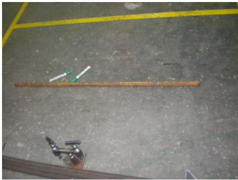
Appendix Figure B1 Dia 20 mm and 32 mm control bars SD40
