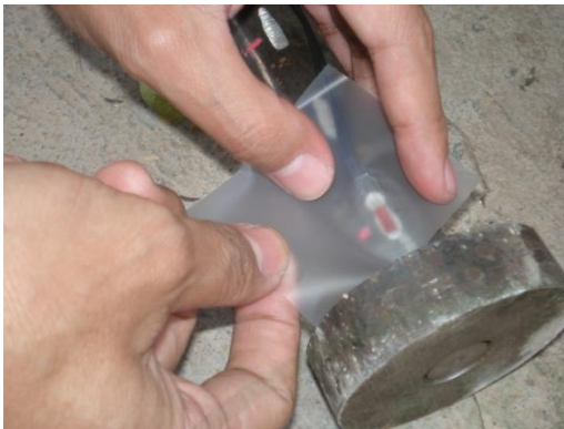
Figure 39 Strain gauges installation along bars
