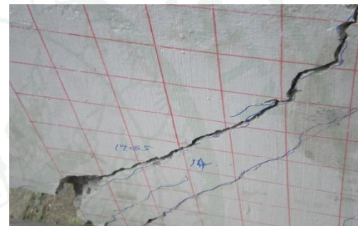
Appendix Figure B32 Cracking behavior for U-20-240-9.59-G-1/1
