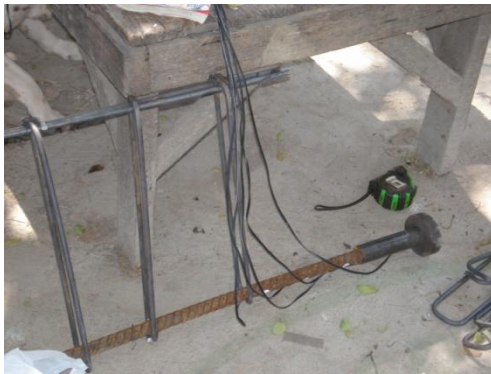
Appendix Figure B16 Strain gauge installation along bars
