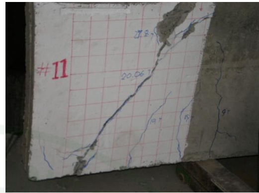
Appendix Figure B40 Cracking behavior for U-20-320-9.59-G-1/1
