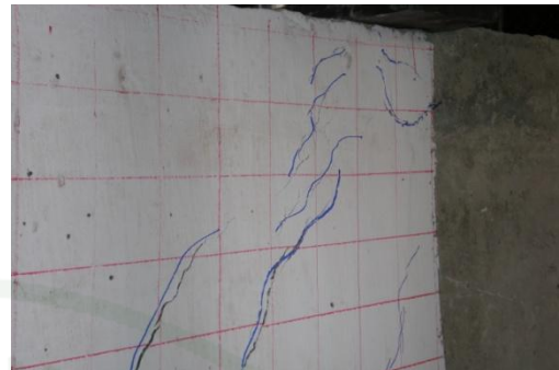
Appendix Figure B31 Cracking behavior for U-20-240-4.32-B-1/1
