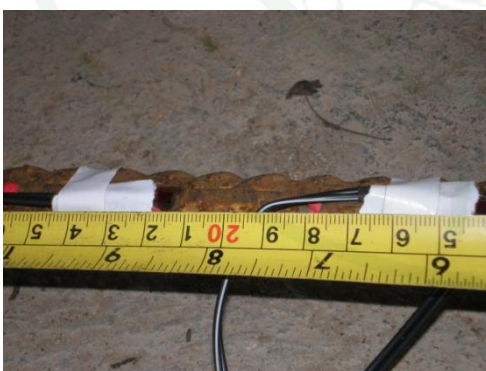
Figure 41 Strain gauges installation along bars
