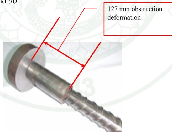
Figure 83 Obstruction deformation of Griptec headed bar
