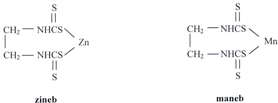
Figure 7 The chemical structure of zineb and maneb
