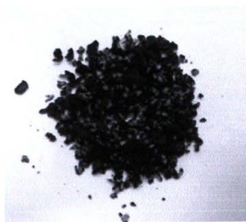
Figure 3.18 The prepared Klason lignin of cassava rhizome
