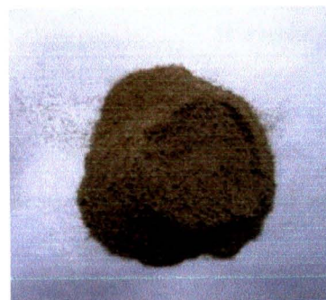
Figure 3.8 Extractive - free jatropa trunk
