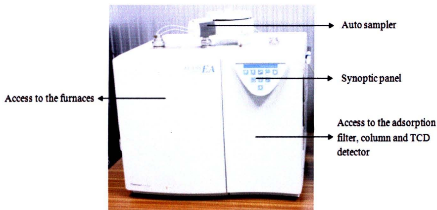
Figure 3.5 A CHONS analyzer used in this study (Thermo Finnigan, Flash EA1112)
