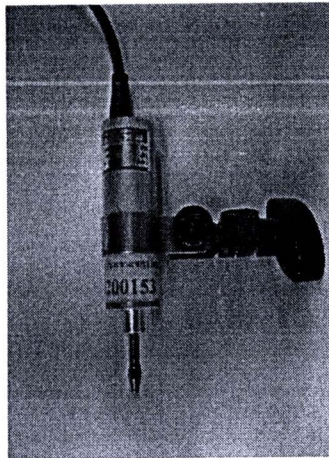
Figure 3.12 LVDT having capacity of 10 mm for global vertical displacement measurement
