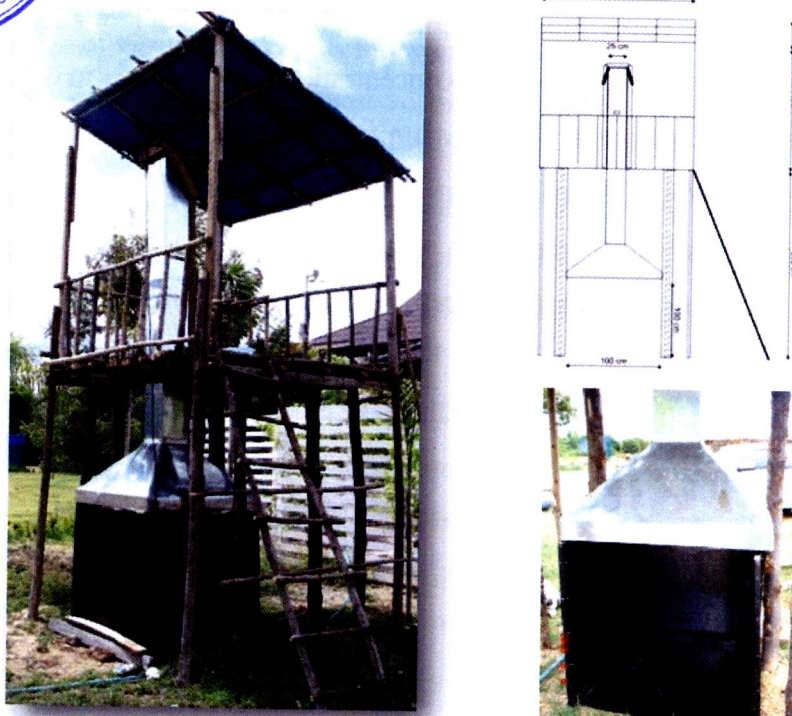
Figure 4.1 Chamber of simulate open burning at KMUTT, Ratchaburi Campus.
