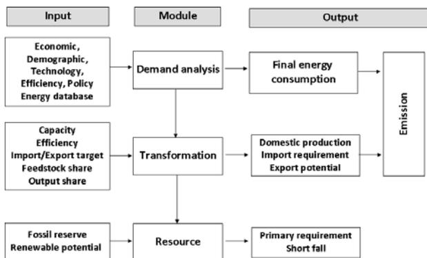
Figure 1 Calculation structure
