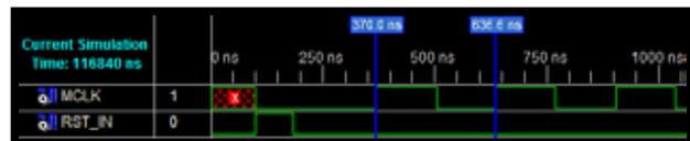
Figure 16. Results of generating MCLK Signal.
