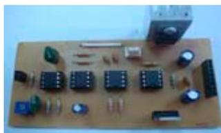
Fig. 4 Circuit board of ECG amplifiers with high pass filter and low pass filter
