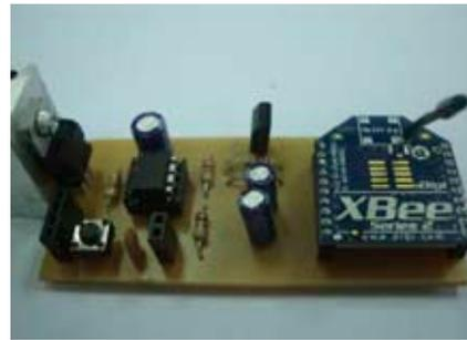
Fig. 5 Microcontroller with ZigBee's transmitter
