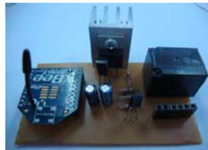
Fig. 6 ZigBee's receiver
