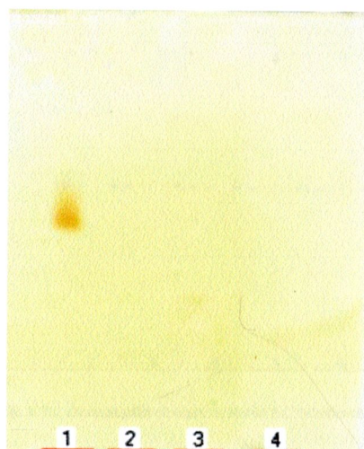
Fig. 1. A TLC of SH (track 1) and synthetic compounds, phenamine (track 2), fenfuramine (track 3) and methamphetamine (track 4) at 10 µg/spot.
