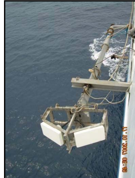
A sketch of mounting Multibeam echosounder at port side.
