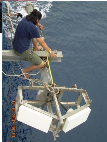
A sketch of mounting Multibeam echosounder at port side.
