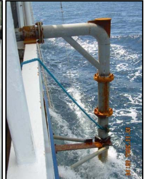
A sketch of mounting Multibeam echosounder at port side.
