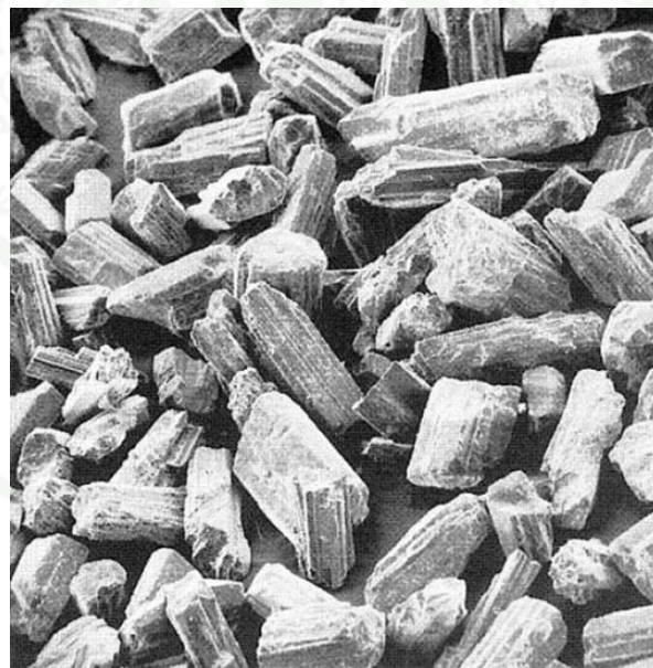
Figure 3 Powder particles of dental stone ( \alpha -hemihydrate). Crystals are prismatic and more regular in shape than those of plaster. ( \times 400 ).
