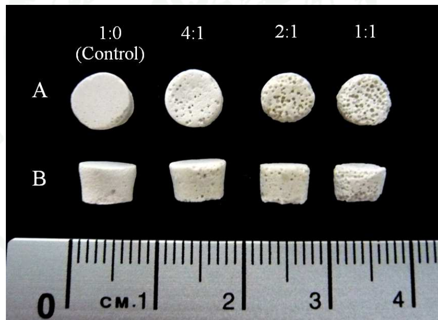
Figure 7 Calcium sulfate beads of various porosities after salt leaching technique: Top view (A); and Side view (B) after mixing calcium sulfate hemihydrates with sodium chloride at ratios of 1:0 (control), 4:1, 2:1 and 1:1 from left to right, respectively.
